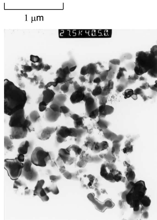
Fig. 2. TEM micrograph of the CR15 powder after milling for 40 h.
